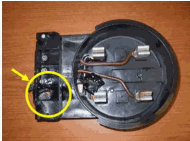
Loose lug on base plate caused arcing
